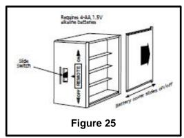
Set the same code combination, as used in the transmitter's code switches above, in the receiver, by using the receiver's code switches. Move the slide button to the "REMOTE" position (Figure 26) and place the receiver in front corner of the fireplace as far from the burner as possible.
