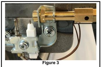
The angle of the pilot flame touching the thermocouple, as set by the factory, is very important to maintain. The alignment and orientation of the ODS pilot is slightly different when the burner is equipped for Natural or Propane gas sources (Figure 4). This should be checked periodically while the pilot is on.
