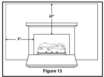
These dimensions are <u>MINIMUM CLEARANCES</u> to maintain when you install this burner system. The fireplace opening <u>MUST BE AT LEAST 6"</u> from any combustible sidewall. The ceiling <u>MUST BE AT</u> <u>LEAST 42"</u> from the top of the fireplace opening.
