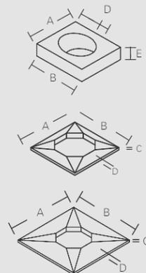
**Please Note:** The DM54 Chimney system is zero clearance to combustible materials. Offset Blocks offer the ability to move a vertical chimney from side to side, allowing it to pass objects above the firebox. Offset blocks require 1 1/2" clearance to combustible material. "Combustibles" are defined as "normal construction materials" and are considered to be: wood framing materials, particle board, mill board, plywood sub-flooring, plywood paneling and wood flooring.
