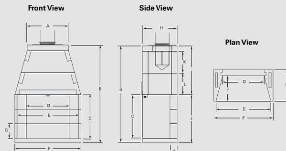
**Please Note:** Different height options are available for the Bvetto fireplace. One additional sidewall and two additional backwalls can be added to obtain an opening of 42" tall before brick is installed. Two additional backwalls and four additional sidewalls can be added to obtain an opening of 52 1/2" tall before brick is installed. Only Isoflames log sets can be used in this unit.
