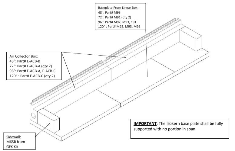
3) The Air Collector Box Assemblies will be placed on top of the base plate(s) as shown (Figure 10).
