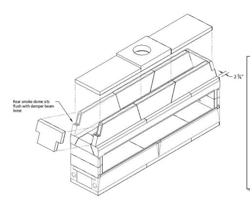
**NOTE:** The underside of the M77 top plate has a stop ledge to seal the smoke dome; the top side is flat.
