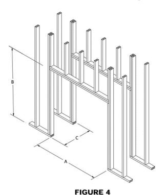
TYPICAL INSTALLATION FRAMING DIMENSIONS
