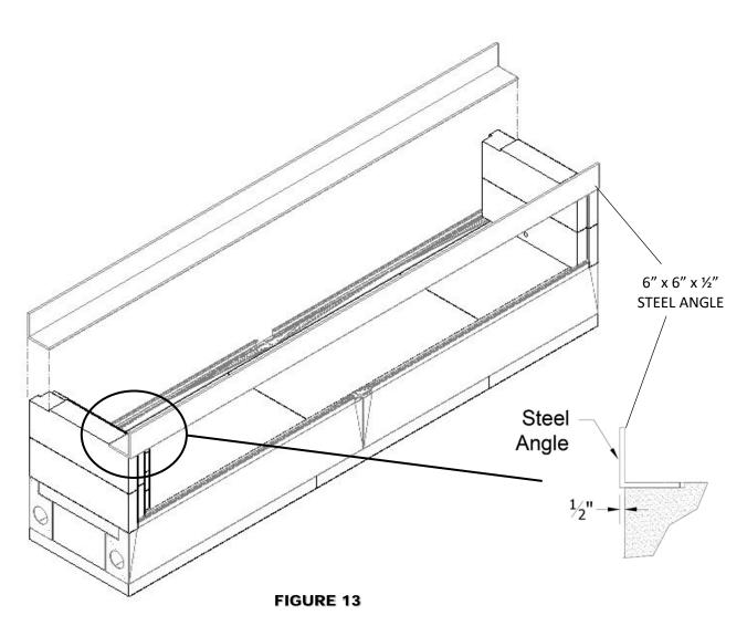
8) The fireplaces come with an 8"- thick damper beam assembly, a component group that is to be assembled on top of the firebox side walls and steel angle iron (no steel angle iron in 48" model). The damper beam assembly consists of long lintel pieces and two (2) short damper end blocks. The lintels will be equal to the width of the fireplace model that they serve. These components both sit on their narrow base so that their beveled face points down and into the firebox interior (Figure 14).
