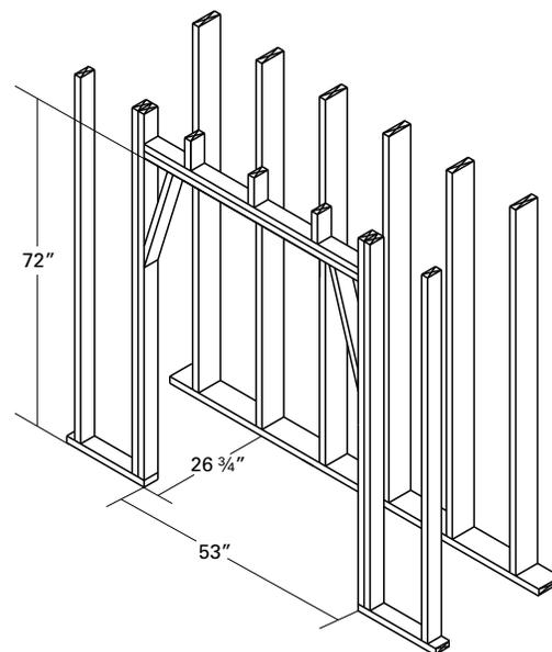
Framing dimensions maintain 1 1/2" clearance to combustibles. This is the standard framing height for the model shown. Refer to product manual for other framing height openings and further installation instructions.
