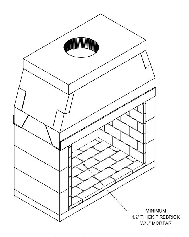
NOTE: IN ORDER TO SUPPORT THE SMOKE DOME OF THIS FIREBOX, A STRUCTURAL STEEL SUPPORT FRAME MUST BE DESIGNED AND APPROVED BY A STRUCTURAL ENGINEER. SMOKE DOME WEIGHT EXCLUDING MORTAR AND EXHAUST COMPONENTS 648 LBS.
