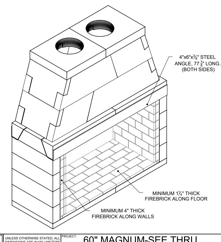
60" MAGNUM-SEE THRU DIMENSIONS ARE IN MILLIMETERS UNSPECIFIED TOLERANCES TO COMBUSTIBLE CONSTRUCTION
