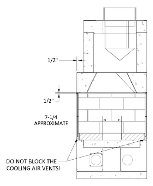
1) Lay two courses of "full" sized firebrick so that the leading edge of the coursing begins at the Brick Barrier that is affixed to the Air Collector Box (s). Ensure a gap of approximately ½" is kept between firebrick and sidewall to allow for expansion.
