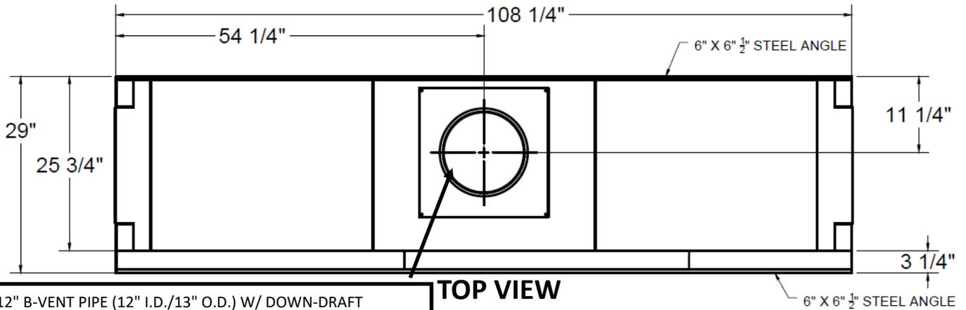
12" B-VENT PIPE (12" I.D./13" O.D.) W/ DOWN-DRAFT DIVERTER; X-VENTISO-MERIDIAN FAN SYSTEM REQUIRED.
