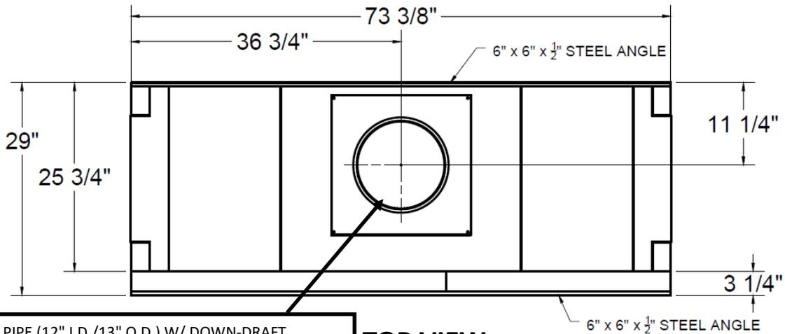
12" B-VENT PIPE (12" I.D./13" O.D.) W/ DOWN-DRAFT DIVERTER; X-VENTISO-MERIDIAN FAN SYSTEM REQUIRED.
