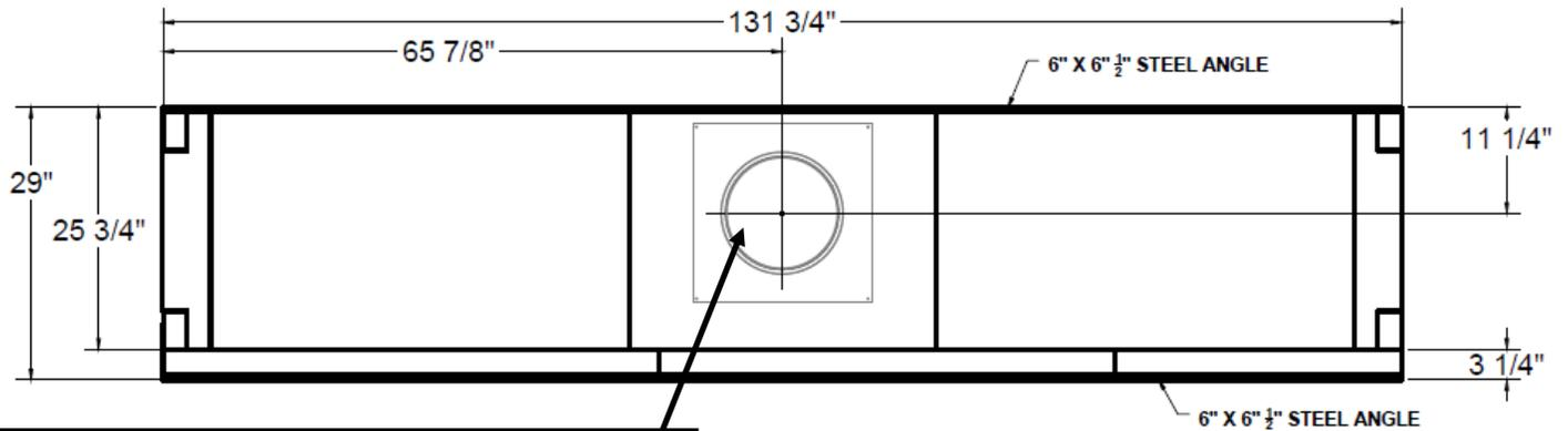
12" B-VENT PIPE (12" I.D./13" O.D.) W/ DOWN-DRAFT DIVERTER; X-VENTISO-MERIDIAN FAN SYSTEM REQUIRED.
