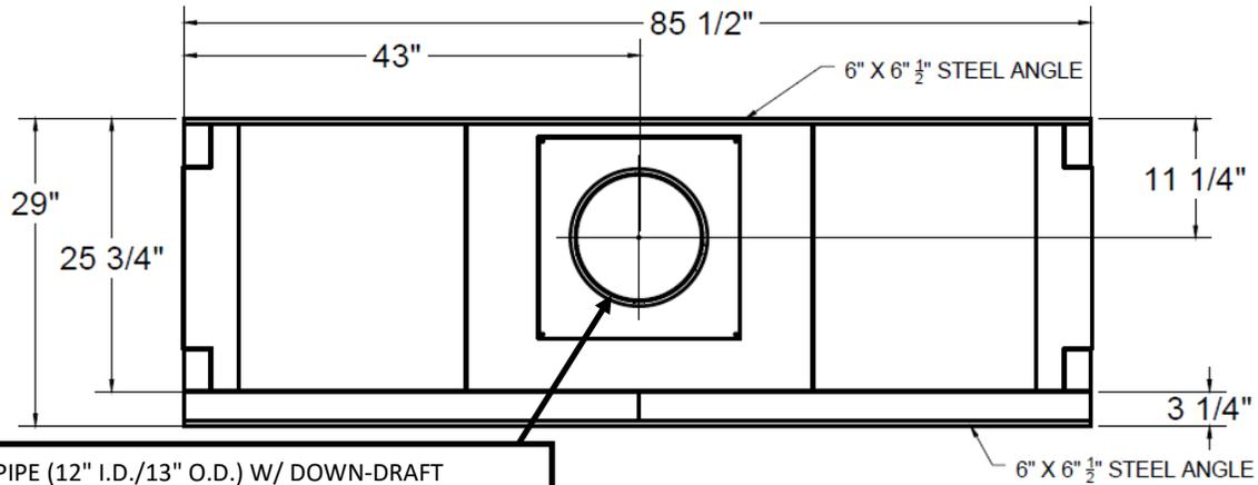
12" B-VENT PIPE (12" I.D./13" O.D.) W/ DOWN-DRAFT DIVERTER; X-VENTISO-MERIDIAN FAN SYSTEM REQUIRED.
