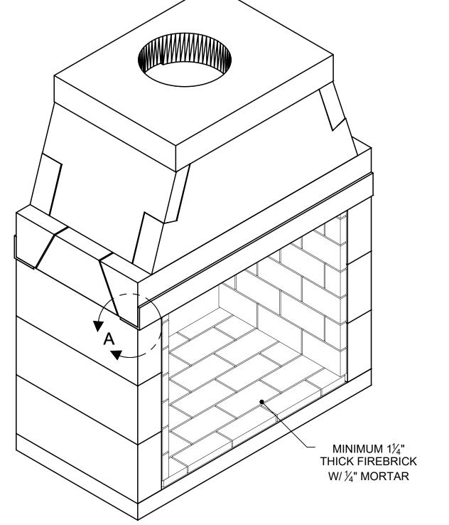
NOTE: WHENEVER THE MAXIMUM DM CHIMNEY HEIGHT OF 57' IS EXCEEDED, OR IN THE FIREBOX/SMOKE DOME ASSEMBLY INCLUDE THE PLACEMENT OF A 4" BY 4" BY 3/8" MINIMUM STEEL ANGLE ACROSS THE FIREBOX OPENING. (SEE DETAIL A)
