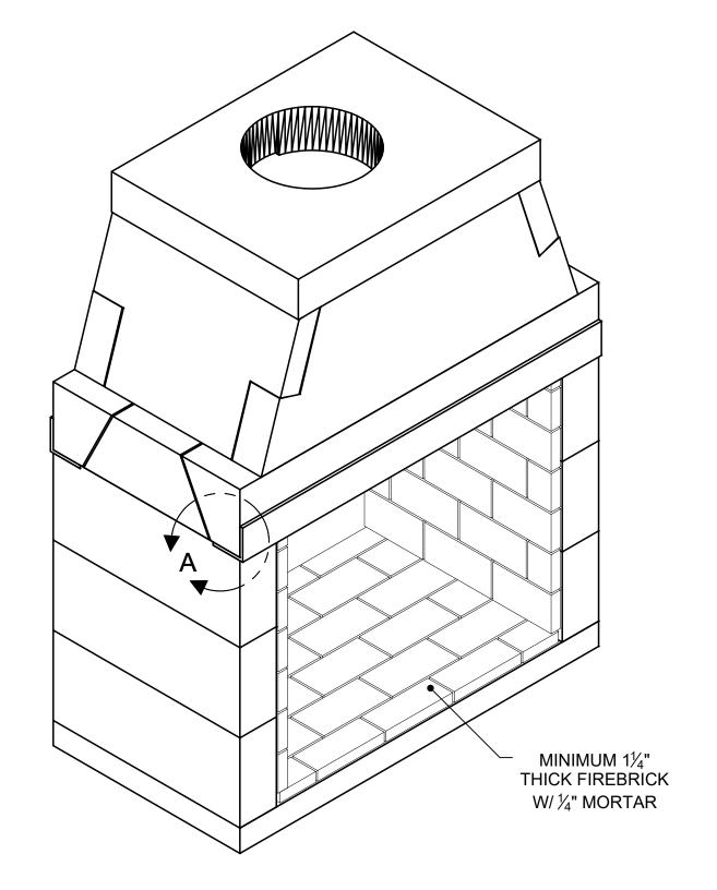
NOTE: WHENEVER THE MAXIMUM DM CHIMNEY HEIGHT OF 57' IS EXCEEDED, OR IN ANY INSTANCE WHERE THE ISOKERN BRICK LEDGE IS USED, IT IS REQUIRED THAT THE FIREBOX/SMOKE DOME ASSEMBLY INCLUDE THE PLACEMENT OF A 4" BY 4" BY 3/8" MINIMUM STEEL ANGLE ACROSS THE FIREBOX OPENING. (SEE DETAIL A)
